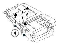
When raising the seatback(s), make sure the lever is locked and you hear the seat latch into place.
